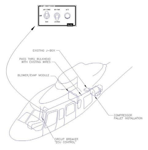
Figure 1. Air Conditioning System General Arrangement
