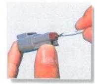
3. Push contact straight into connector grommet until a click is felt. A slight tug will confirm that it is properly locked in place.
