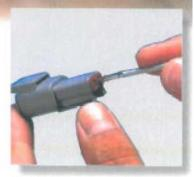
3. Hold the rear seal in place, as removing the contact will displace the seal.
