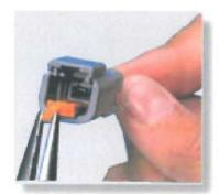
Remove orange wedge using needlenose pilers to pull wedge straight out.
