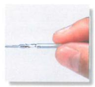
Grasp crimped contact approximately 1.0" (25.4mm) behind the contact barrel.
