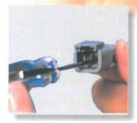
To remove the contacts, gently pull wire backwards, while at the same time releasing the locking finger by moving it away from the contact with a screwdriver.
