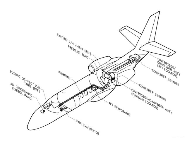
Figure 1. Air Conditioning System General Arrangement
