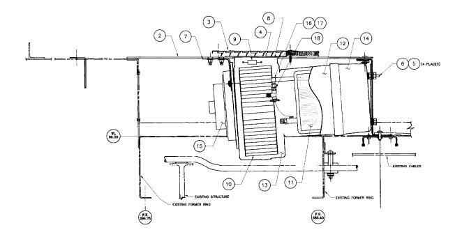
Figure 1. Aft Evaporator Assembly
