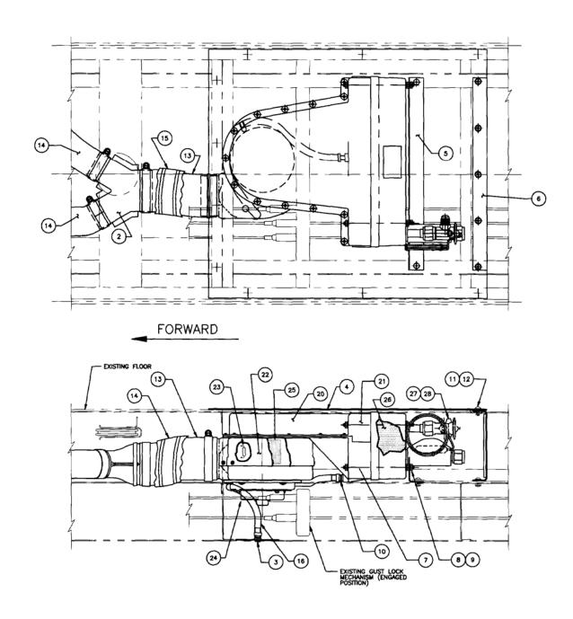
Figure 2. FWD Evaporator Assembly (Cool Stick Option)
