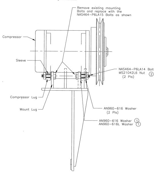
1) Install washers as required to fill space between lugs. Normally one AN960-616 Washer on each side will be adequate, but due to the variation in thickness of the washers you may need one AN960-616 and one AN960-616L to fill the space between the lugs and mounting ears, see details.
