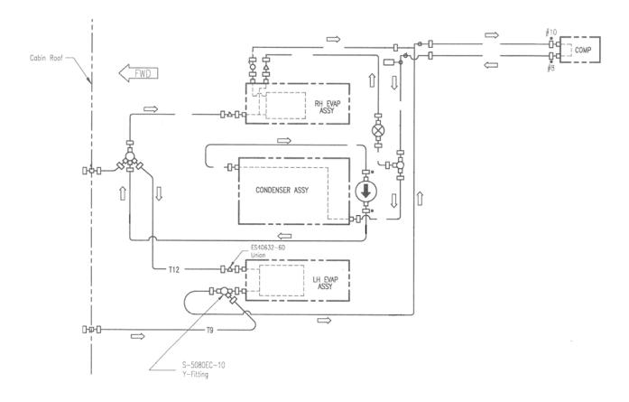
Figure 10: Dual Aft Evaporator Plumbing Schematic
