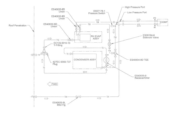
Figure 13: Single Aft Evaporator Plumbing Schematic
