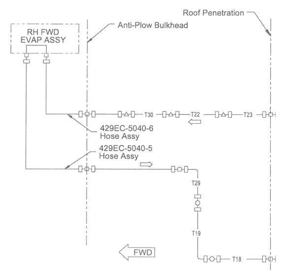
Figure 6: Single Forward Evaporator Plumbing Schematic
