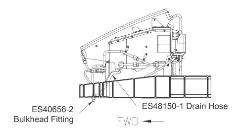
Figure 8: View of Left Aft Evaporator Assy Looking Inboard from LH Side
