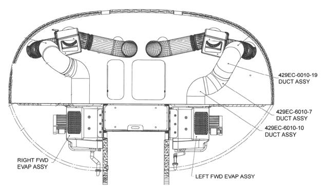
Figure 3: View Looking Aft at Fwd Evaporators and Ducting
