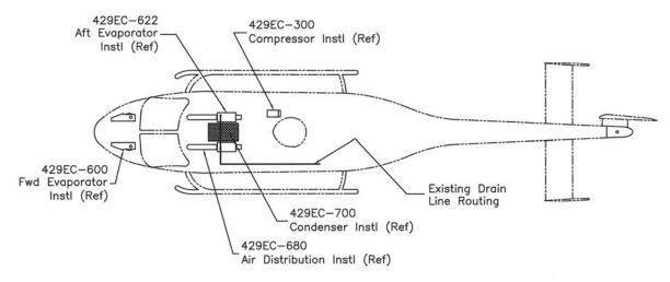
Figure 1: 429EC-200; General Arrangement – 429 Dual A/C System
