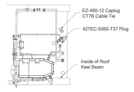
Figure 9: Top View of FWD Flight Control Deck (Condenser Not Shown)
