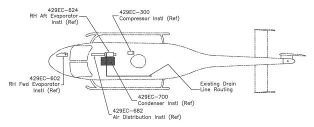
Figure 2: 429EC-202; General Arrangement – 429 Single Fwd/Aft Evap A/C System
