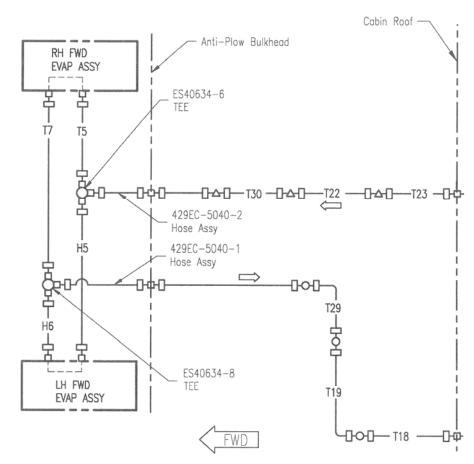
Figure 4: Dual Fwd Evaporator Plumbing Schematic
