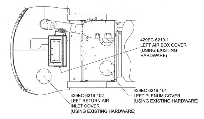
Figure 12: Single Aft Evaporator Air Distribution
