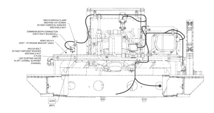
Figure 16: LH Aft Evap Connector ACP8 Stowage Bracket Details
