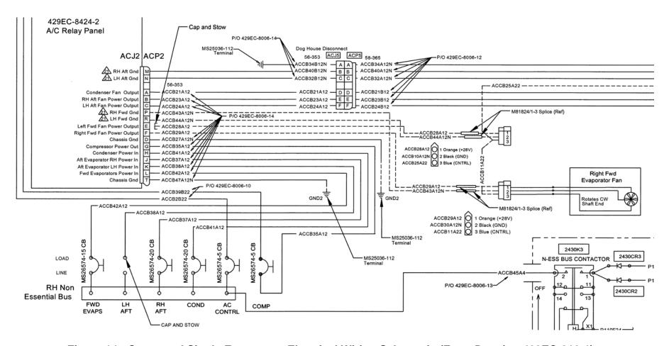
Figure 14: Converted Single Evaporator Electrical Wiring Schematic (From Drawing 429EC-812-1)
