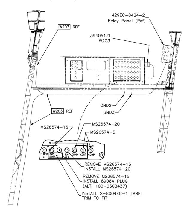
Figure 15: Circuit Breaker Change Details
