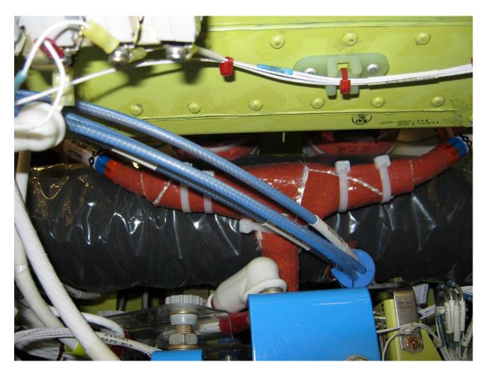
Figure 7: Firesleeve over defroster Tee fitting and heater tube.
