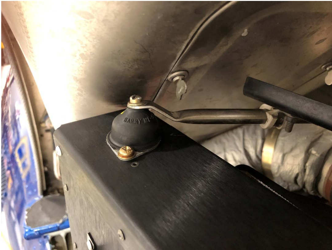
Figure 1: Typical bending of EC145-7016-12 Support Tube
