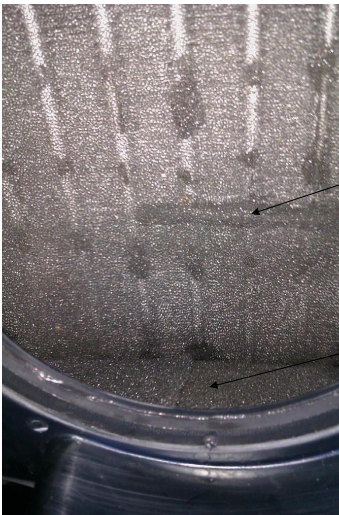
Figure 30: ES04122-1 and 429EC-6242-1 Water Screens shown in place. View looking forward through blower opening
