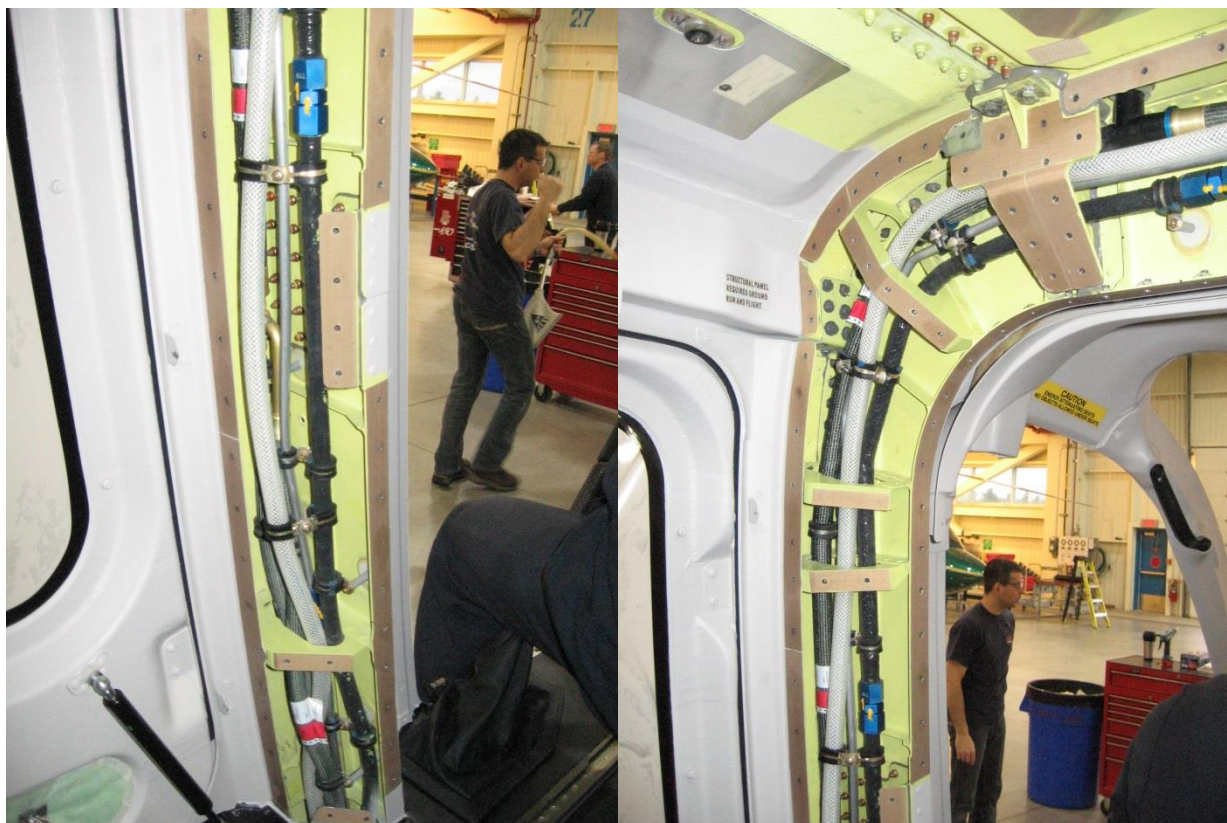
Figure 24: Drain Hose routing in left door post showing clamping arrangement
