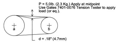
Figure 2: Belt Tension Inspection
