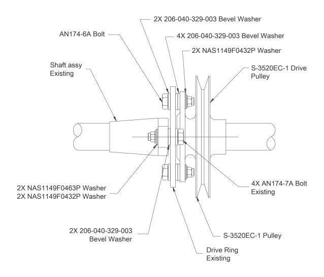
Figure 6: Detailed View of Compressor Pulley
