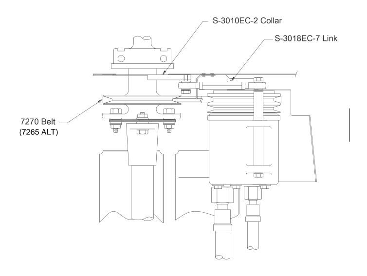
Figure 7: View of Compressor Drive
