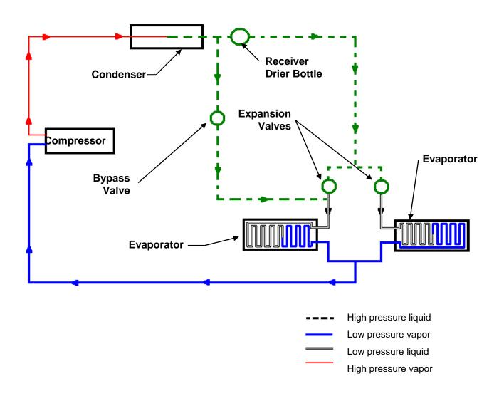
Figure 1: Refrigeration Cycle Illustration
