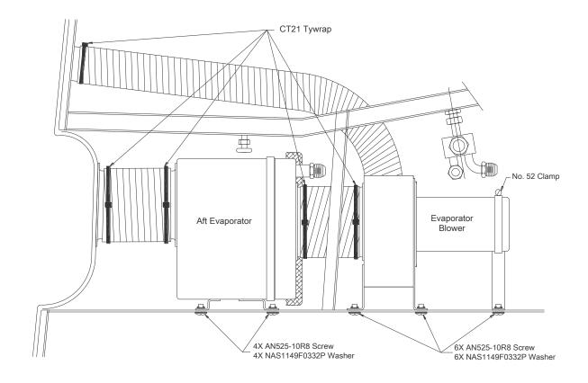
Figure 14: Evaporator Blower - VIEW E-E
