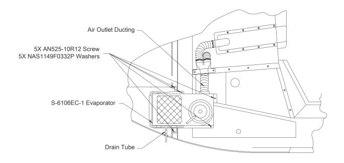
Figure 13: Forward Evaporator - View G-G
