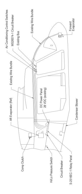
Figure 9: Electrical system components
