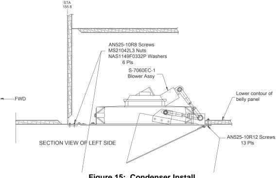
Figure 15: Condenser Install
