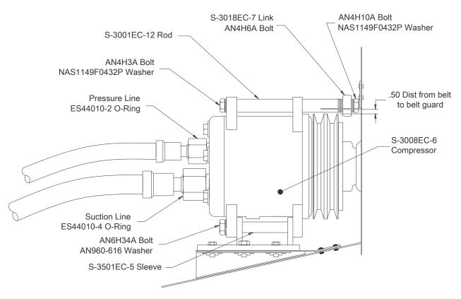
Figure 11: Compressor - View D-D
