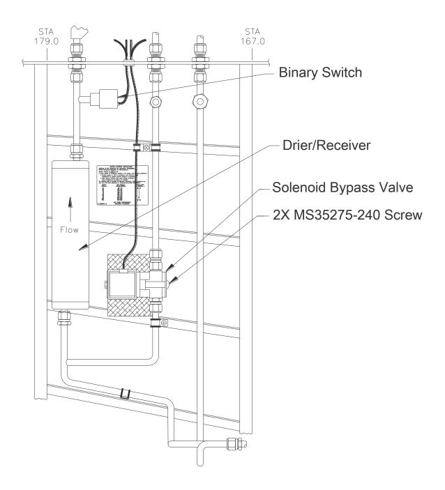
Figure 18: Binary Switch - View F-F
