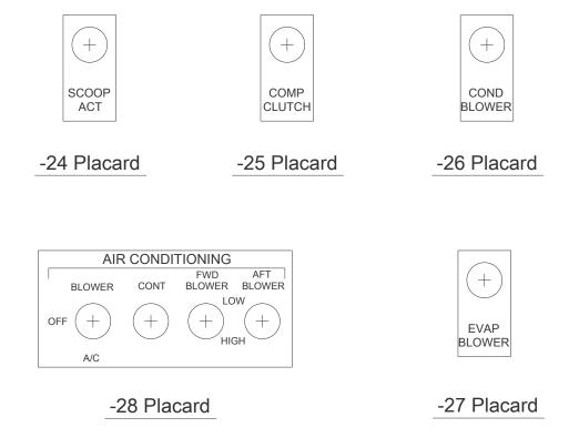
3. The above placards must be displayed adjacent to the appropriate circuit breaker or switch on the overhead circuit breaker panel in the cockpit.
