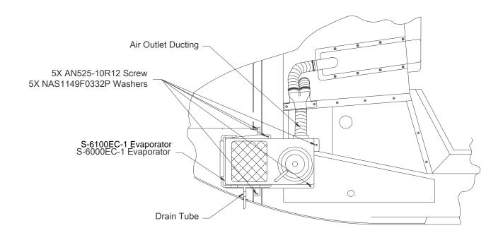
Figure 13: Forward Evaporator - VIEW G-G
