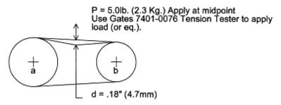
Figure 2: Belt Tension Inspection
