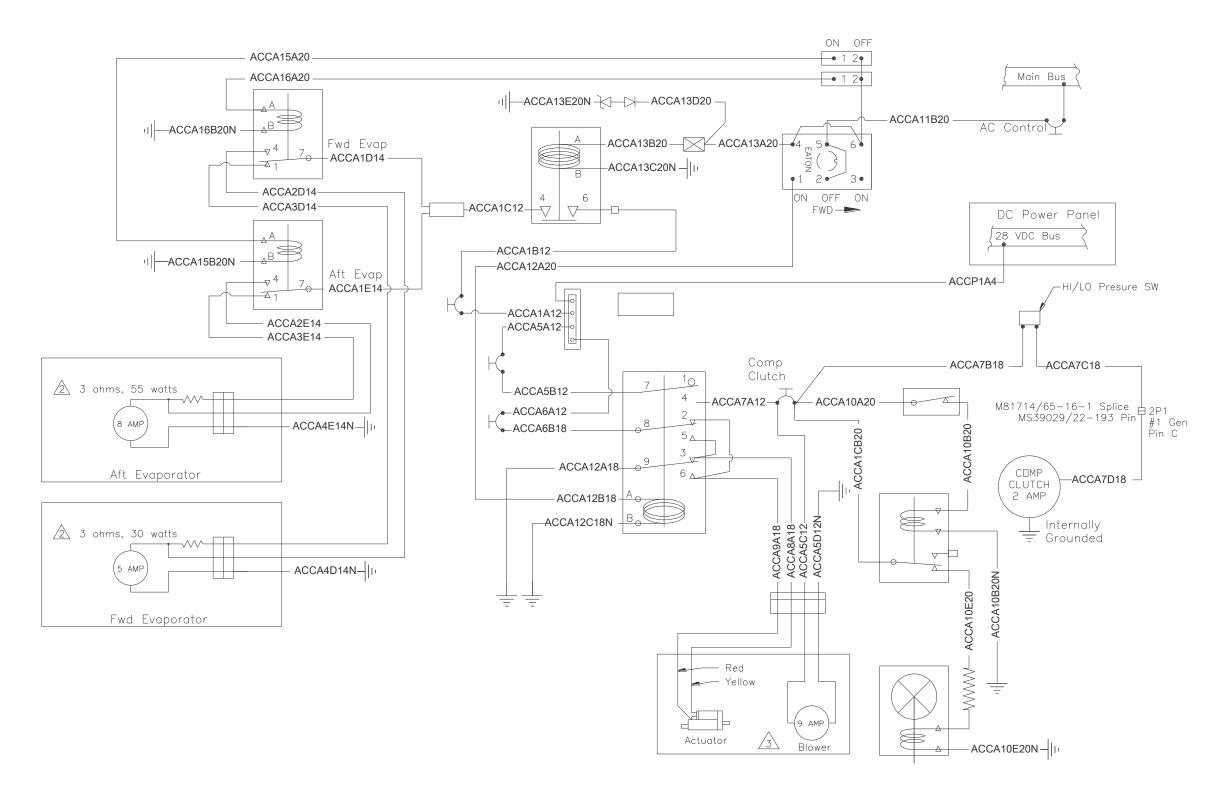
Figure 19: Electrical Schematic
