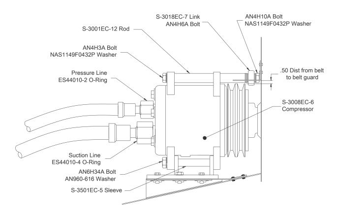
Figure 11: Compressor - VIEW D-D
