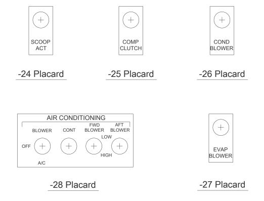
2. The above placards must be displayed adjacent to the appropriate circuit breaker or switch on the overhead circuit breaker panel in the cockpit.
