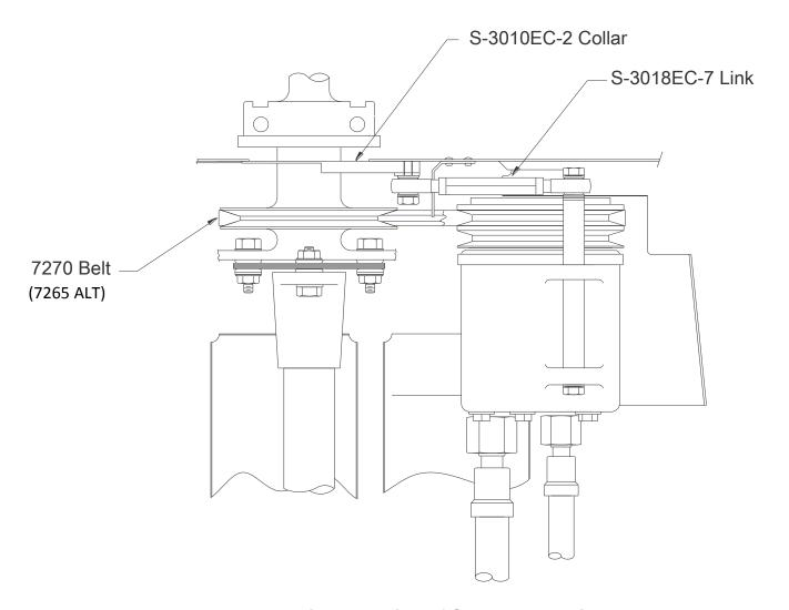
Figure 7: View of Compressor Drive
