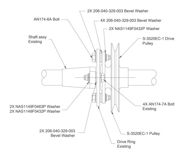
Figure 6: Detailed View of Compressor Pulley
