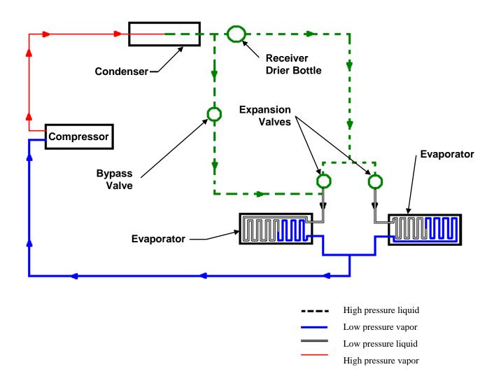
Figure 1: Refrigeration Cycle Illustration
