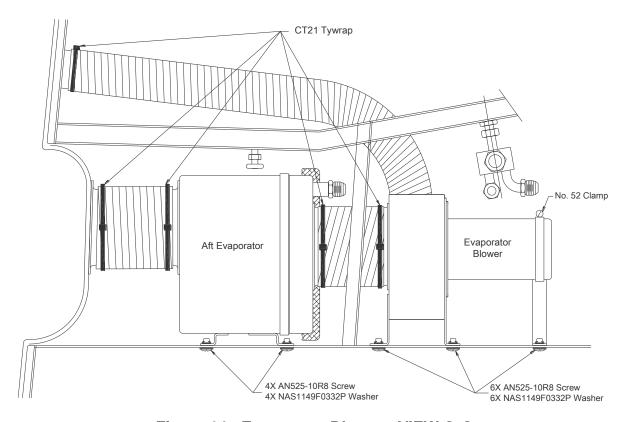
Figure 14: Evaporator Blower - VIEW G-G
