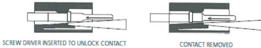
Figure 5: Molex pin removal
