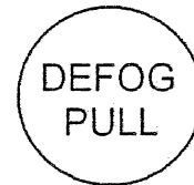
Figure 6. Defog push-pull cable: located pilot/co-pilot sides adjacent to inboard air outlets
