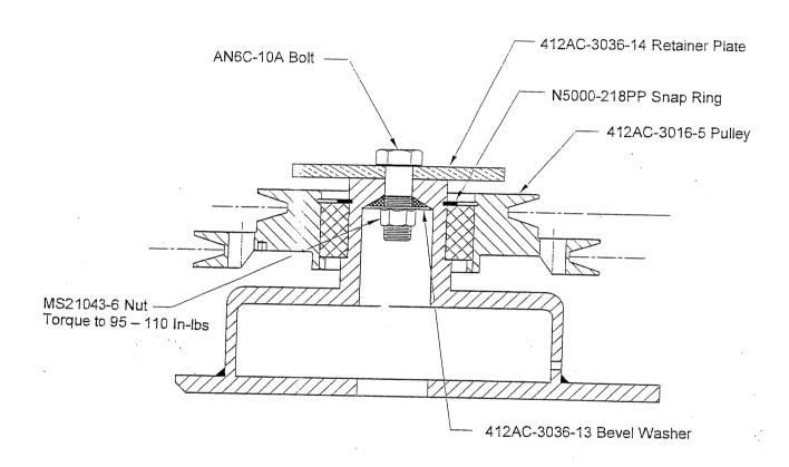
Figure 1, 412 Air Conditioner Speed Reducer Assembly
