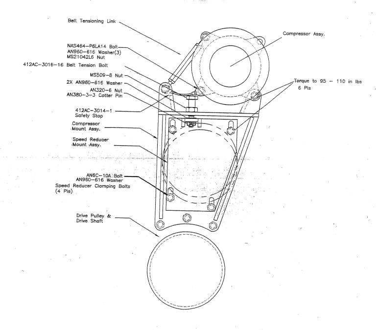
Figure 2, 412 Air Conditioner Compressor Mount and Speed Reducer Assembly
